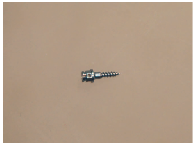
Figure 2. Tested miniscrew: 1.6 \times 7 mm (Turkuaz, TasarımMed, Istanbul, Turkey).
